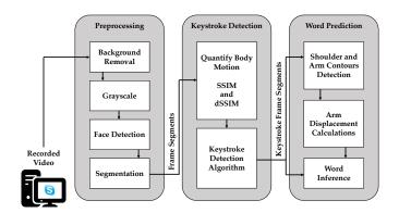
Fig. 1: Overview of the keystroke inference framework.
