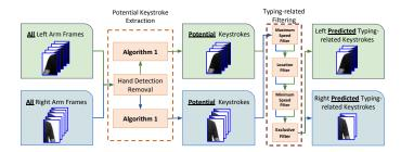
Fig. 3: Overview of the typing activity detection technique.
