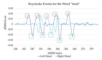
Fig. 2: An example of  $dSSIM^{L^s}$  during a typed word. Circles represent the actual keystroke event, whereas squares represent the local minima within two frames of every keystroke.
