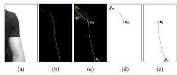
Fig. 4: (a) A keystroke frame segment, (b) Outer contour (OC), (c)  $45^{\circ}$  projection from  $p_{\alpha}$  that intersects OC at  $p_{\beta}$ , (d) Shoulder contour (SC), and (e) Arm contour (AC).
