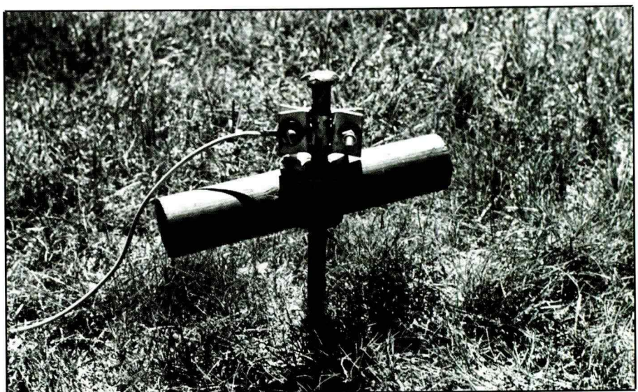
Fig. 2. Be sure to provide some way to remove your ground stake, like the cross-piece shown at the top of the stake in this photo, in case it must be relocated.
