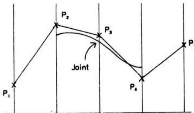
Another section of curve can be generated using points  $P_2$ ,  $P_3$ ,  $P_4$ , and  $P_5$ . The two curved pieces will be connected with  $c^2$  continuity at the joint. The equation to generate a section is
