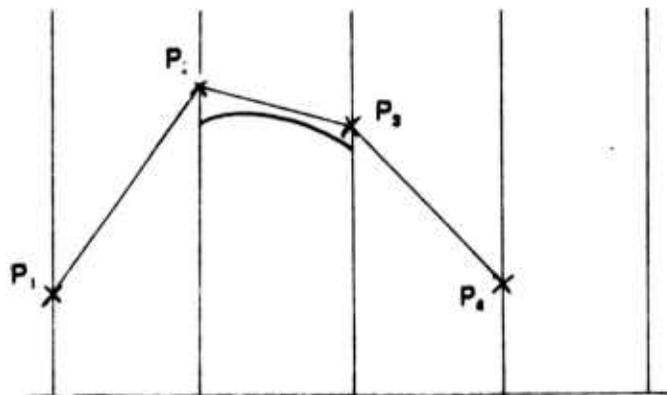
A cubic curve can be generated that in general does not pass through any of its four control points. Now consider a fifth point  $P_5$ .
