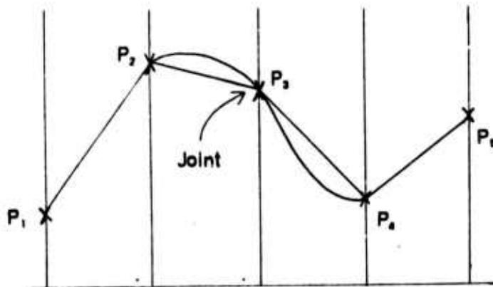
Another piece of curve can be generated using points  $P_2$ ,  $P_3$ ,  $P_4$ , and  $P_5$ . The two sections will be connected with  $C^1$  continuity. The equation to generate a section is:
