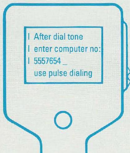
Fill in the computer's telephone number if it isn't already shown. Put a pound (#) between digits to indicate a 2-second pause in dialing where required (to wait for a second dial tone behind a PBX number, for example). For a longer pause, press pound (#) several times.
