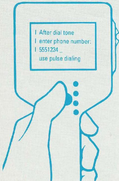
When the correct phone number is shown, move the Pointer to the right side (anywhere along the right side will do) and press. If you need to rotary dial, select the last line with the Pointer before you press. The Craft Access Terminal will dial the number. You can redial by moving the Pointer to the right side and pressing again.
