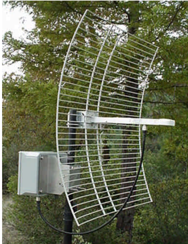
Figure 25: Mounting of Parabolic Grid 24 dBi Gain Antenna (Horizontally Polarized)
