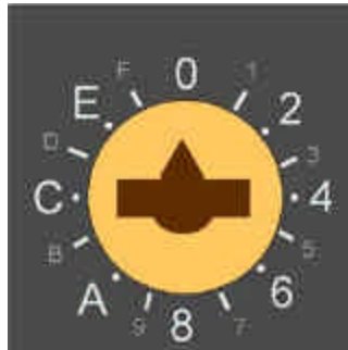
Figure 7: Rotary Switch Identification with Channel 0 setting shown
