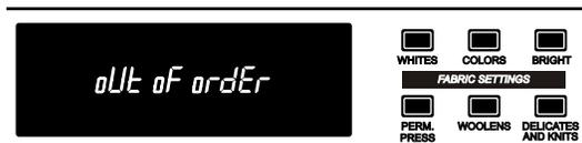
**NOTE:** Not displayed on washer as shown. Message scroll followed by the failure code.
