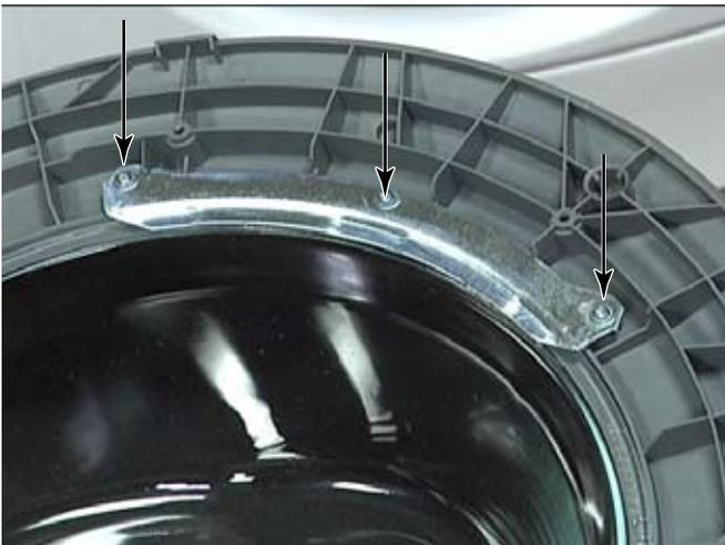
10. Support the inner door trim to avoid having it drop when removing the bowl brackets.
