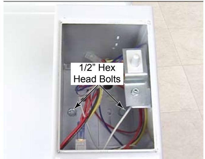
6. Remove the metercase from the washer and the pad that is between the metercase and the washer top.
