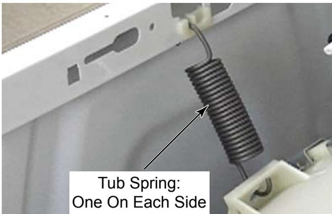
**NOTE:** To avoid damage to components in the cabinet base or on the outer tub, do not let the tub drop free inside the cabinet.
