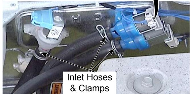
7. Remove the T-20 screw, on the back of the washer, that secures each water inlet valve.
