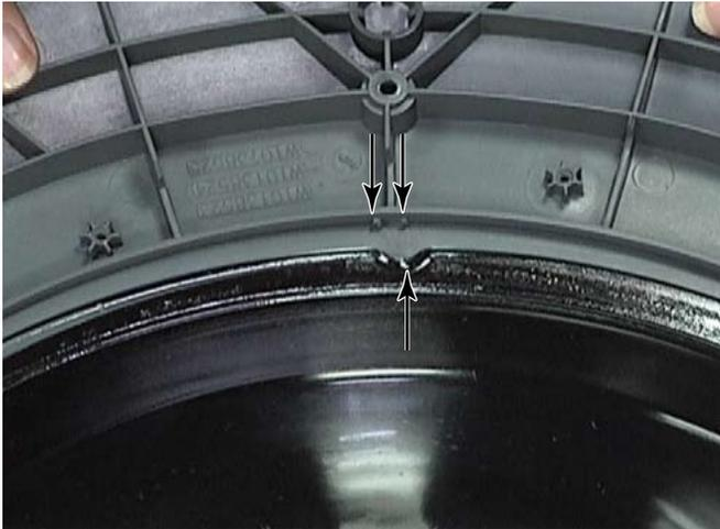
12. There is no gasket or sealing material between the inner door panel and the bowl. The bellow seats and seals against the glass of the bowl which should keep water from reaching this area. This is why the glass bowl needs to be cleaned periodically to avoid build up of hair and debris which will cause water leakage through the door seal.
