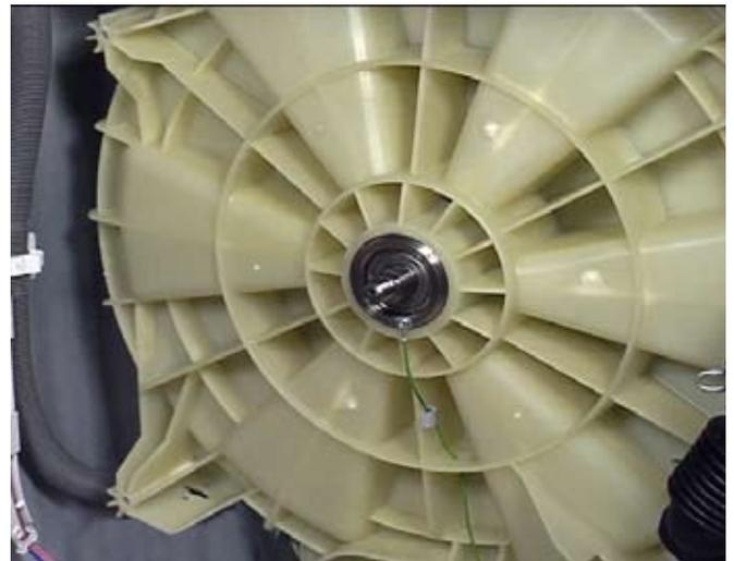
**NOTE:** When reinstalling the 15/16" nut make sure it is tightened to between 50-60 foot pounds. If not tightened sufficiently the washer may produce knocking noises that sound like a failed bearing.
