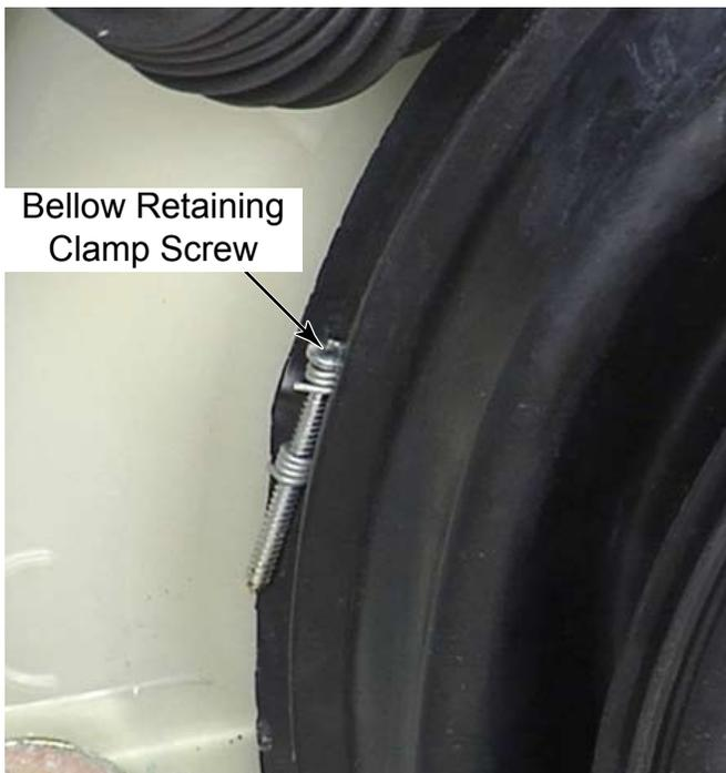
5. Remove the bellow retaining clamp from around the bellow.
