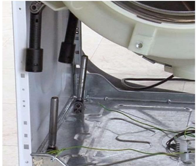
20. If replacing the tub, remove the six flat nuts that secure the weights to the tub by prying them out of their slots with a flat blade screwdriver. Flat nuts are usually not supplied with a replacement tub.
