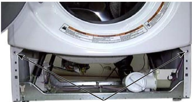
7. Remove two 1/4 inch hex head screws, that were hidden by the control panel cover, that secure the top of the front panel to the washer side panels.
