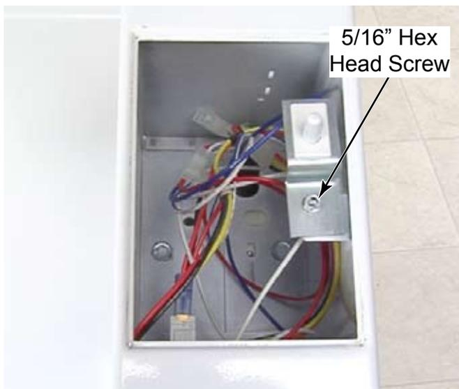
4. Remove the switch, bracket and wire harness.
