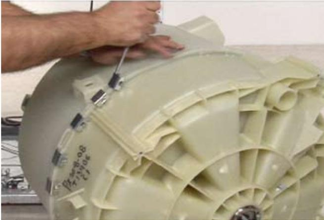
23. Press the tab on 2 of the 3 guides around the edge of the tub to release the tub halves. The 3 guides will assist in re-aligning the tub halves during reassembly.
