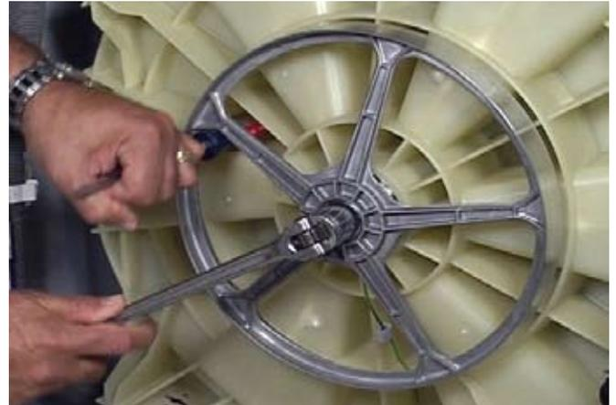
6. Pull the pulley off the shaft.
