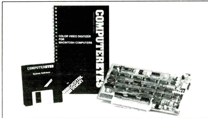
board and software on 3.5-inch diskette. The system captures high-resolution images by acquiring  $640 \times 480$ -pixel samples for display on either 8- or high-resolution 24-bit display systems. Images can be captured from any standard video source, including any NTSC composite or S-video source. It captures monochrome or color images with 8 or 24 bits of color information per sample for near-photographic quality imaging.
