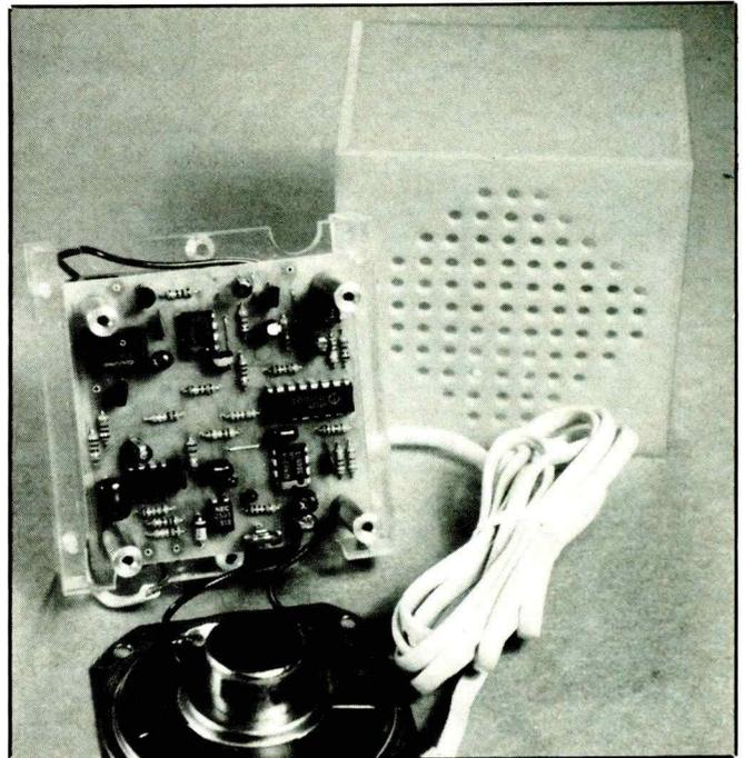
In reality, the Super Tunes circuit does not distinguish between incoming ring pulses and outgoing dial pulses on the line. Instead, it disables the ability of the triggering circuit to turn on the melody-producing section while the phone is off-hook. This prevents the melody from playing every time you pick up the phone to dial a number.
