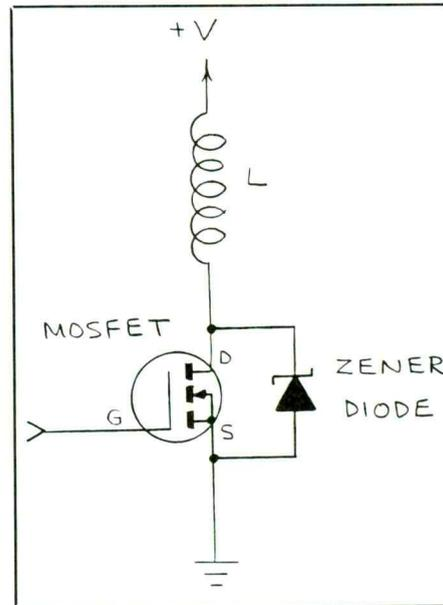
Fig. 3. Protecting a MOSFET with a zener diode clamp.
