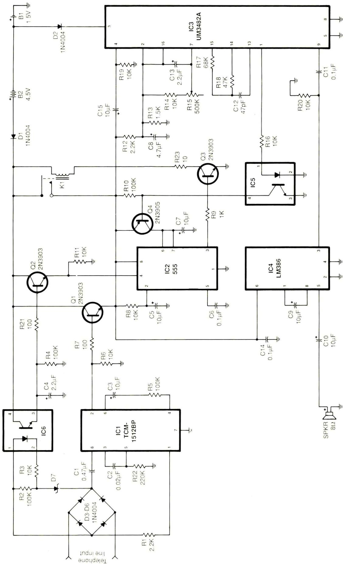
Fig. 1. Complete schematic diagram of Super Tunes telephone melody ringer circuitry.
