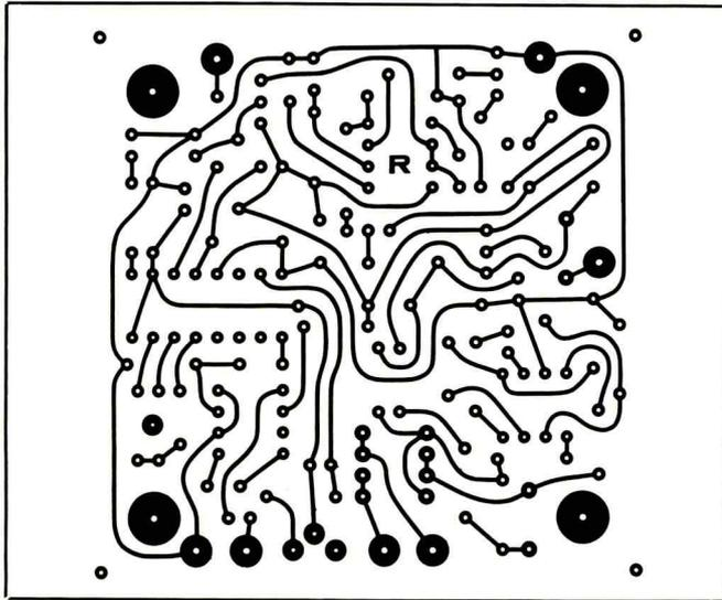
Fig. 2. Actual-size etching-and-drilling guide for fabricating printed-circuit board.
