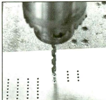
Fig. 5. Tip of No. 27 drill ground almost flat removes circle of copper for both terminal pins and IC pins.
