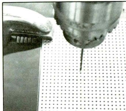
Fig. 4. To ensure that IC sockets fit properly, clamp piece of perforated board with holes on 0.1" centers to pc blank to serve as drilling guide.
