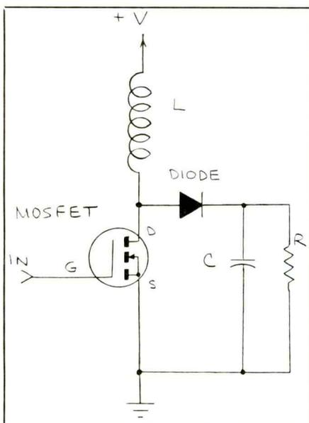
Fig. 4. Protecting a MOSFET with a snubber network.
