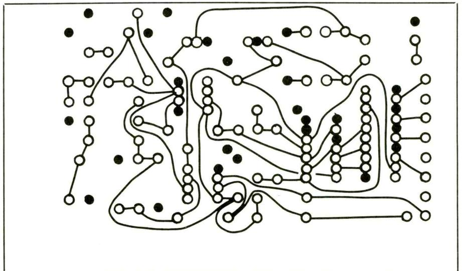
Interconnections are made using bus wire and sleeving (photo). If proper pins and sockets are employed you can use Wire Wrap techniques. Wire runs and soldering points are illustrated in drawing (solid black dots indicate points soldered to copper cladding).
