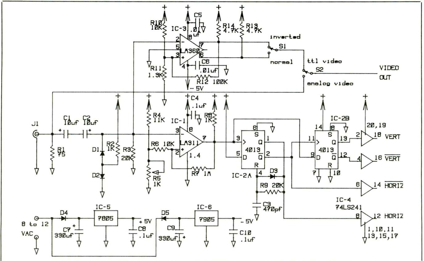
Fig. 2. Complete schematic diagram of circuitry used in Non-Composite Video Adapter. Only component not shown is ac power transformer, which can be a plug-in wall-type unit.
