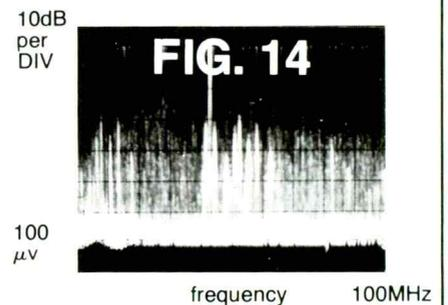
Wrong. Fig. 14 shows the effect of a drill operated on the same line. Momentary RF levels exceed the 70dB probe overload range. Even an SCR light dimmer puts out interference. Arcing insulation in an AC motor will exhibit high levels of "trash" — observable as significant change in line RF when energized. A thunderstorm is a real experience!
