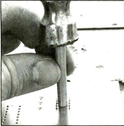
Fig. 6. After all holes are drilled and terminal pads are cleared of copper, IC sockets install by pounding them into place on board.
