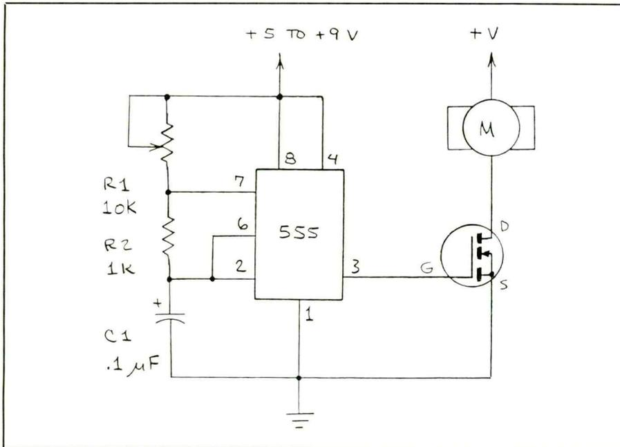
Fig. 7. Power MOSFET motor speed controller.
