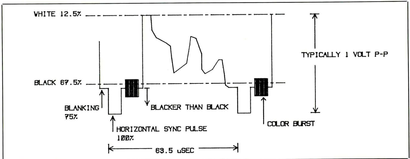
Fig. 1. Composite video signal consists of video, blanking and sync pulses.
