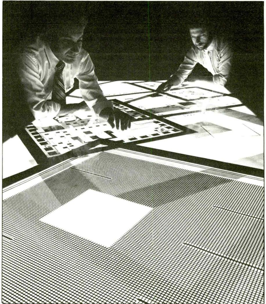
Fig. 1. Mask pattern for a power MOSFET made from thousands of parallel-connected transistors. (Courtesy IXYS Corporation.)
