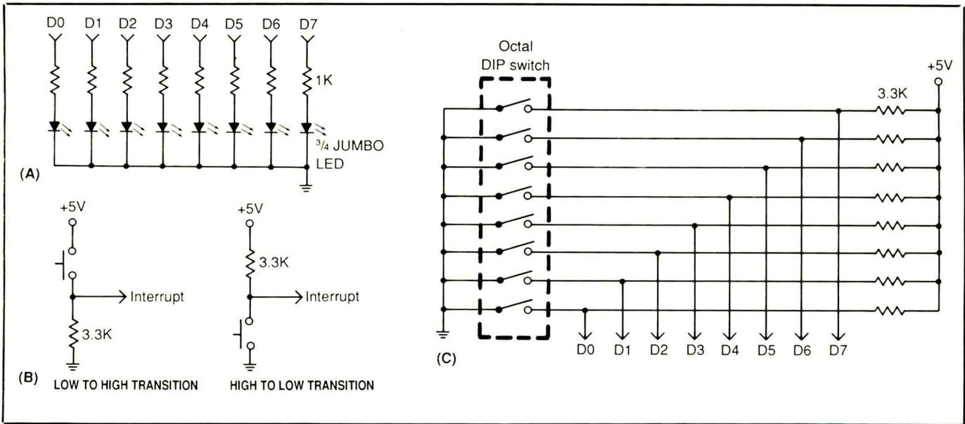
Fig. 3. Example of LED array (A) that can be used to exercise output port. One array is shown; three arrays are required in full implementation. Momentary-contact pushbutton switches (B) can be used to exercise interrupt inputs. One of two DIP-switch assemblies (C) that can be used to exercise the input ports.
