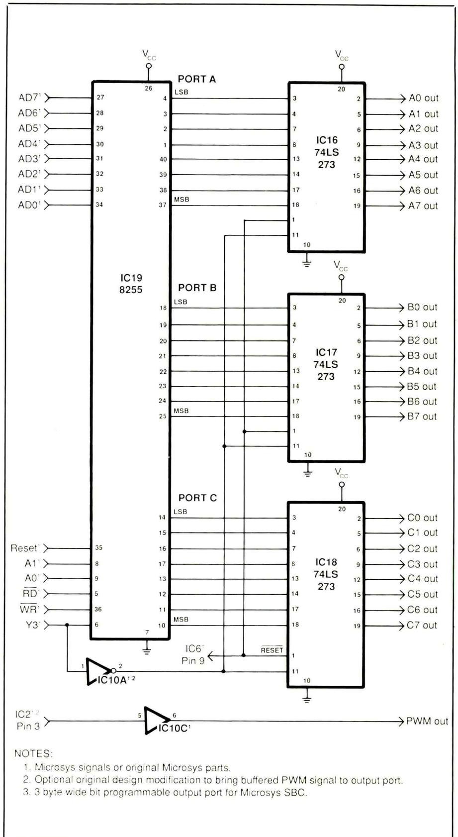
Fig. 2. Output circuitry details.
