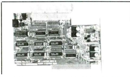
series or compatible computer. It buffers the computer from harm and allows the pc card under test or development to be removed or inserted without having to power-down the PC or affecting its operation.
