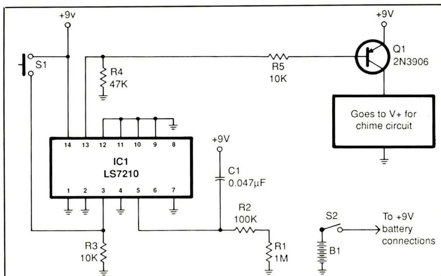
Fig. 1. Schematic diagram of Delay section of the Infinite Snooze Alarm.
