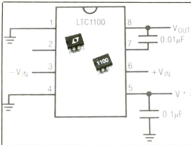
Linear Technology's LTC1100 chopper-stabilized instrumentation amplifier has less than  $2 \mu\text{V}$  of error and less than  $2 \text{ nV}/^\circ\text{C}$  offset drift.
