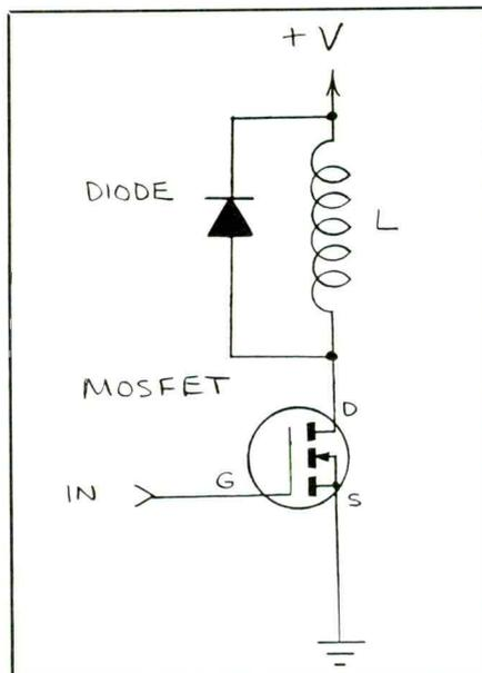
Fig. 2. Protecting a MOSFET with a diode clamp.
