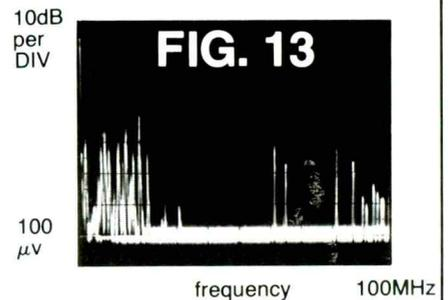
The high voltage rating of the Spectrum Probe<sup>®</sup> input isolating capacitance allows direct connection to the power line. (Don't connect to the power line unless you are knowledgeable and can meet U/L requirements!!!) The incoming power line RF was observed between line and ground (through a GFI for insurance) in Fig. 13. It would seem to make a good antenna.
