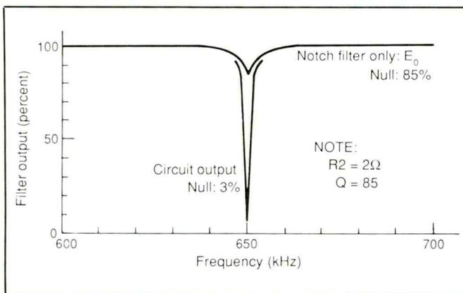
Fig. 5. Depth-of-notch improvement of typical notch filter circuit.
