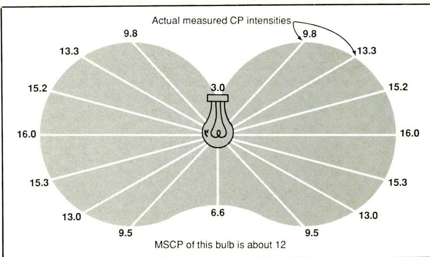
Fig. B. Luminous intensities in different directions of an incandescent lamp. MSCP of this lamp is about 12. This data was adapted from *American Electrician's Handbook, Ninth Edition*.
