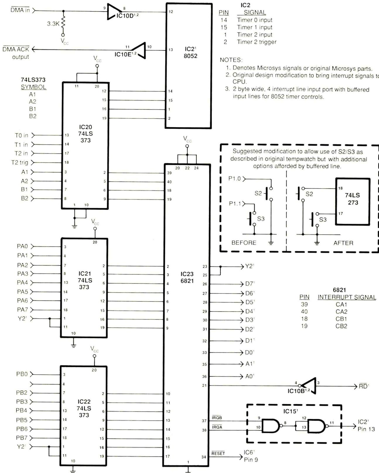
Fig. 1. Input circuitry details.
