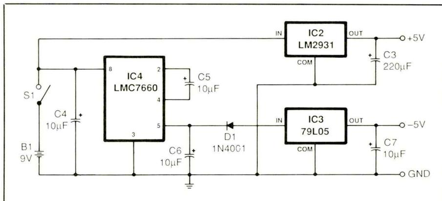
Fig. 3. Schematic diagram of power supply used with both versions of project.
