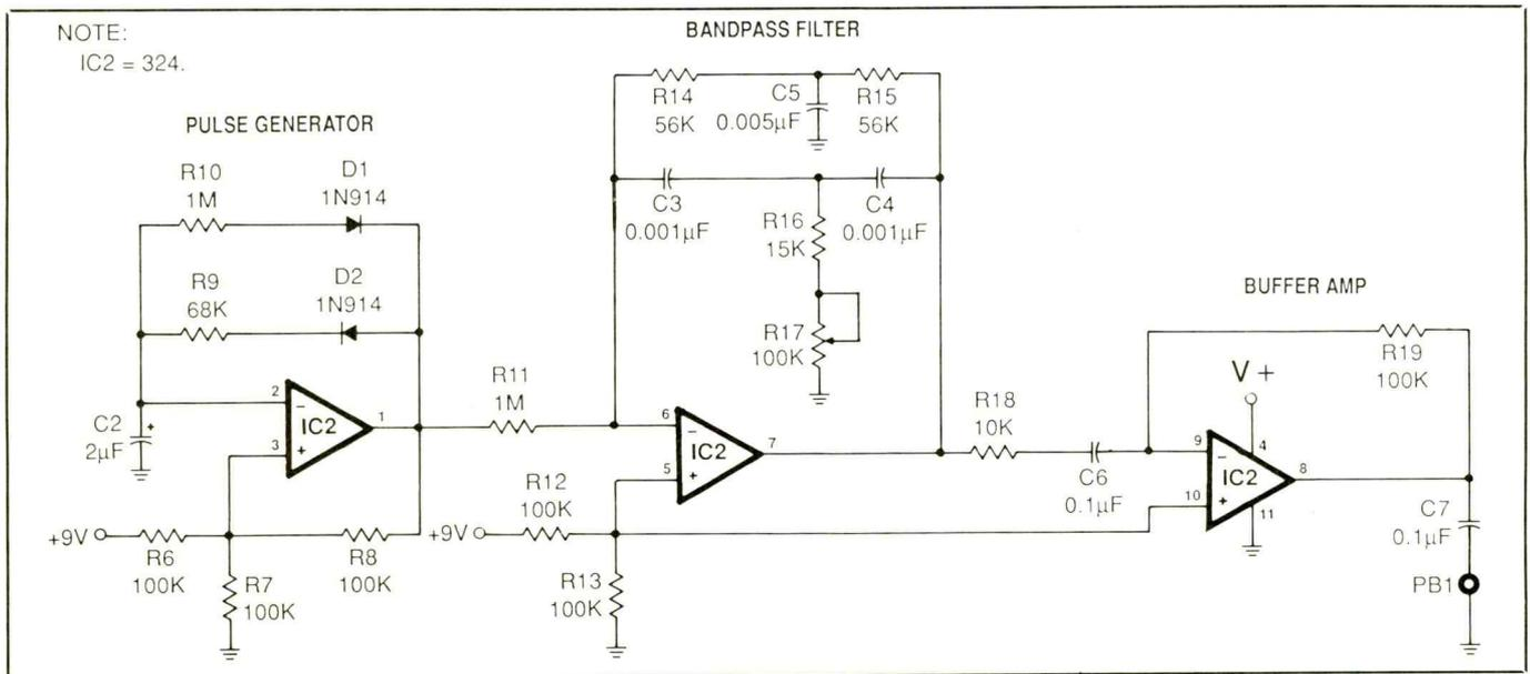
Fig. 2. Schematic diagram of Chime section of project.
