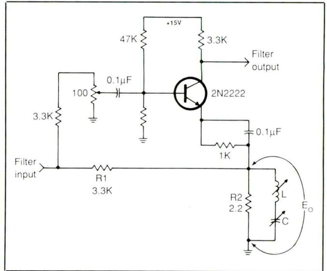
Fig. 4. Schematic diagram of a typical notch filter circuit.
