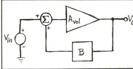
In the above diagram,  $A_{vol}$  and B are the gains of the amplifier and feedback network, respectively. Notice that  $V_1 = BV_o$ ;  $V_2 = V_{in} + V_1 = V_{in} + BV_o$ ; and  $V_o = V_3 = A_{vol}V_2$ . Substituting the expression for  $V_2$  in the last equation, we get  $V_o = A_{vol}(V_{in} + BV_o)$ . Rearranging this last equation, we obtain  $V_o = (A_{vol}V_{in})/(1 - A_{vol}B)$  and  $(V_o/V_{in}) =$
