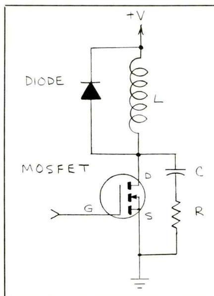
Fig. 5. Modified version of the snubber arrangement in Fig. 4.
