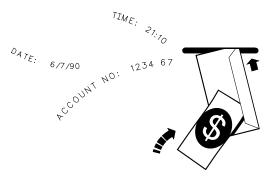
The *personaS*<sup>88</sup> can be fitted with an envelope depository that can accept envelopes with contents up to **12.7 mm** (0.5 in.) thick. A printer built into the depository can print up to 80 alphanumeric characters along the envelope as it is transported to the depository bin. The data printed on the envelope is under application control.
