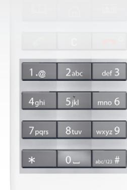
**0-9, a-z, period (.), @, space, \*:** Press a key repeatedly to toggle between the options displayed on each key.
