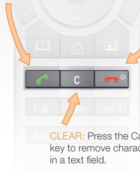
**END CALL, STANDBY:** Press the End Call key to end a call, or when idle, press and hold the key to go into standby mode.
