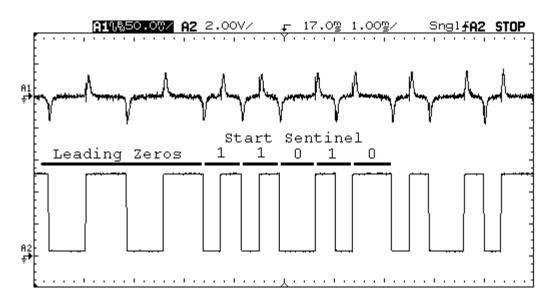
The figure above is a scope shot of the circuit in action. In this particular case, a read head was interfaced directly to an AN10E40. The top trace shows the raw read head input... noise and all. The bottom trace shows the circuit's output
