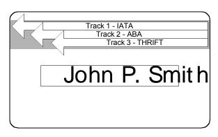
For this discussion, the figure to the left represents the back of a typical plastic credit card. With the magnetic stripe on top as shown, the first (top) track is encoded in a format established by the International Air Transport Association, this track usually has your name encoded on it.
