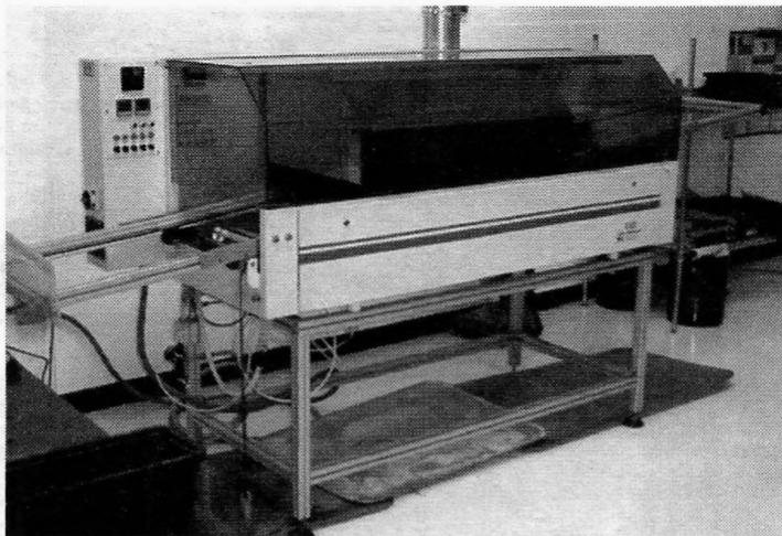
**A typical flow solder machine. It would solder all joints on the pc board at one time, drastically reducing labor costs**
