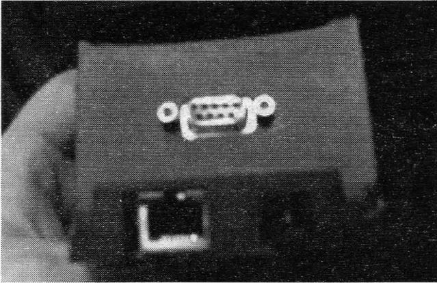
Figure 3. 9-pin in the back so the cradle can still be used with the palm.
