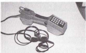
To the left, we have a Harris TS-22 linemans test set pictured. It's also known as a beige box, more or less. Pictured on the right, we have two Progressive Electronics tone generators - the 77M (smaller unit) and the 100A (the larger unit)
