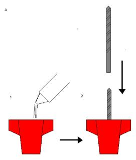
In figure (A) a large electrical romex wire connector is filled (A-1) with hot glue then drill bit is inserted into the wire connector and held till glue cools straight, centered and upright (A-2). Glue in cap should be allowed to sit and harden for at least 8 hr to achieve a strong bond. I use "winged" wire connectors to make
