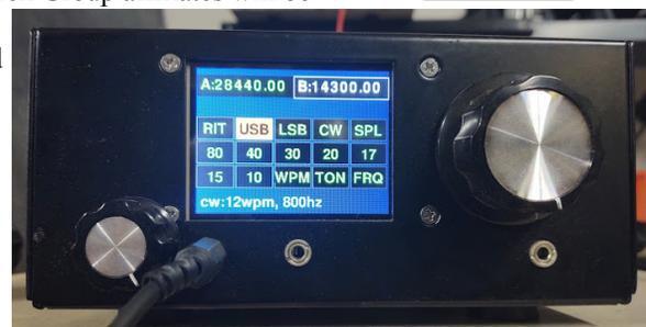
uBITX is a 10 Watt HF Amateur Radio transceiver kit that is Open Source and based on the Arduino Nano (<https://www.arduino.cc/en/pmwiki.php?n=Main/ArduinoBoardNano>). The full kit is \$209. The basic kit (minus speaker and enclosure) is \$160. At those prices, it provides a reasonably-priced alternative to more expensive 10 Watt class HF radios. Being Open Source and Arduino-based, the hacking possibilities for this radio are numerous, and significant hobbyist community support is available.
