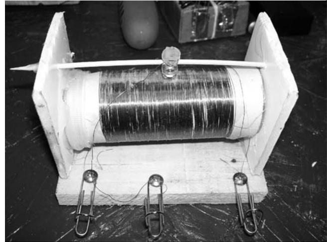
I believe the wire for the tuning coil was either salvaged from a transformer out of a microwave oven, or purchased from our (somewhat) local electronic/industrial surplus store, P&T Surplus in Kingston, NY. It's about an hour and a half drive to get there, but well worth the trip. The coil form is a vitamin bottle.
