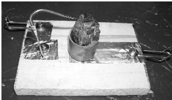
Here we have a picture of the detector crystal. This is the heart of a crystal radio system. The crystal is a piece of Galena purchased at a local rock shop, Nature's Art in Montville, CT. The cat's whisker is
