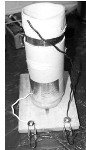
The heart of this capacitor is made from two paper towel rolls covered in aluminum foil and placed one inside the other. He discovered that the performance was less than adequate, so it is being re-designed.
