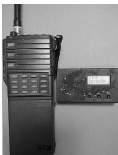
If you have an HT with DTMF capability you already have half of this system. You just need a DTMF decoder to complete it. An inquiry with your favorite search engine will find software that will enable you to decode DTMF tones with your PC's soundcard. Amazon and Ebay have assembled DTMF decoders and kits that are a little smaller than a pack of cigarettes. Most, if not all, of them use the standard 8870 DTMF decoder IC, and will have similar performance.
