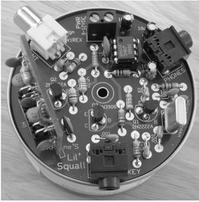
A modern version of the Novice CW HF rig kit is still being made in Maine by W1REX at QRPme. The Lil' Squall costs \$40 and will operate on 80, 40, 30, 20, and 10 Meters. It's an up-to-date version of the famous Tuna Tin QRP radios, so named because the PCB was designed to fit on top of a tuna fish can. The Lil' Squall is all thru-hole solid state discrete components on a PCB board. The parts are all common and easily found. You could get one of the
