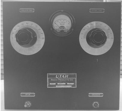
For those of you looking for a holy grail, keep your eyes open for a late 1930's vintage Utah Junior HF CW transmitter. It was sold as a kit for Novice ham radio operators. It has only two tubes: a rectifier and a 6L6. It's crystal controlled and will transmit on all bands from 160 to 10 Meters. The RF output is balanced, so you can home brew the entire antenna system from whatever wire you can find. The output stage is tunable, so no antenna tuner is needed. You simply match
