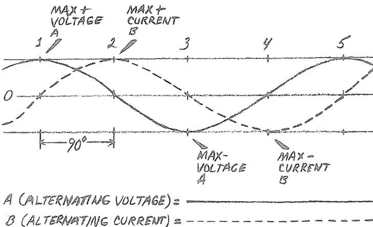
*NOTE ON PRECEDING DIAGRAM: (A and B are said to be ninety degrees out of phase. A "cycle" of current/voltage from peak to peak is 360 degrees. 90 degrees out of phase means that when alternating voltage A is at its peak strength, alternating current B is at zero.)*
