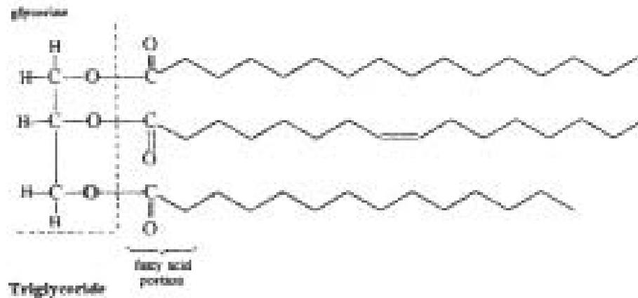
During transesterification a basic catalyst breaks the fatty acids from the glycerin one by one. If a methanol contacts a fatty acid they will bond and form biodiesel. The hydroxyl group from the catalyst stabilizes the glycerin.
