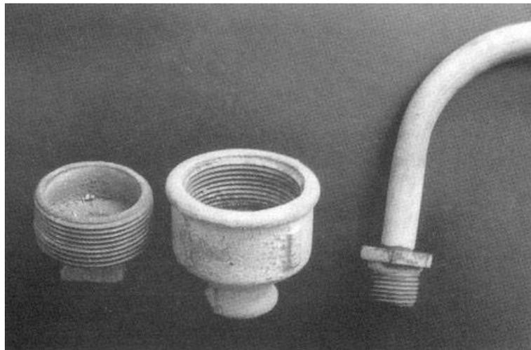
2. Connect the 1;2-inch-to-1 V2-inch (2c to 2b) reducer to the reducing bush by screwing tightly.
