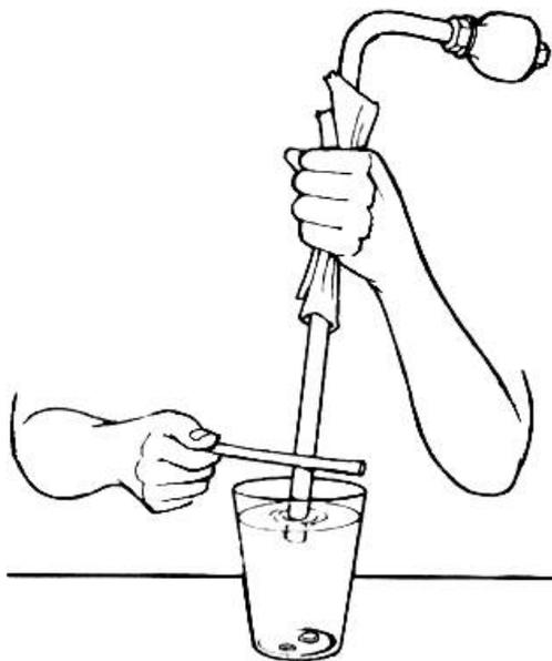
Figure 6: Tap the pipe to remove the mercury
