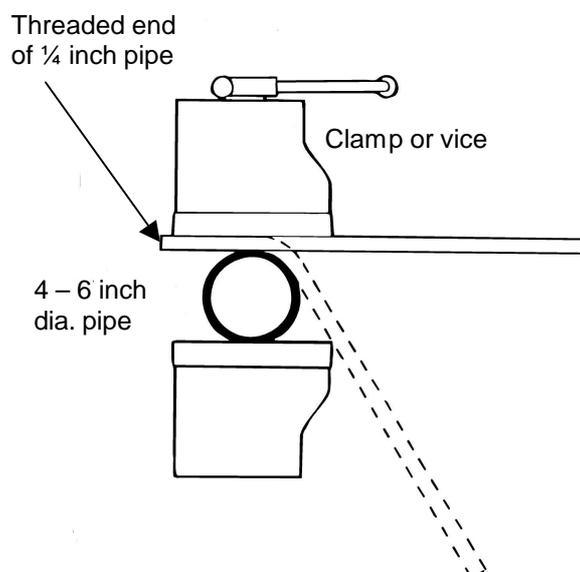
Figure 1: Pipe bending using a clamp or vice
