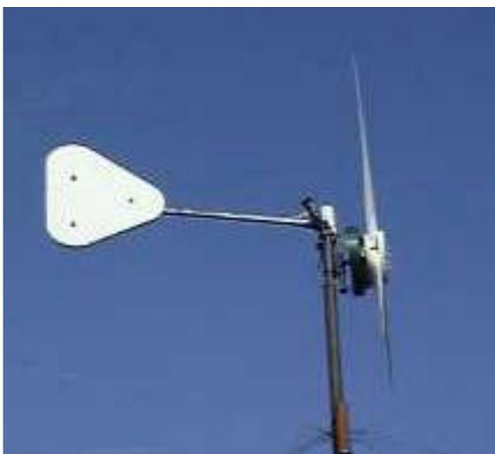
Figure 2: The ITDG wind generator for battery charging © ITDG
