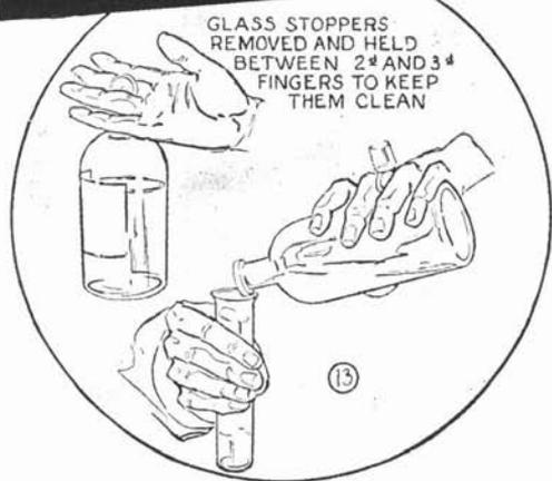
When heating substances in test tubes breakage is avoided by following the suggestions shown in Fig. 11. Fig. 13 shows the proper method of removing stoppers from bottles to prevent their becoming dirty and thus contaminating the contents of the bottle when replaced. When intense heat is required it may easily be produced by directing the flame of a blowtorch into a hole cut in the side of a flowerpot as shown in Fig. 12. It is very convenient for melting metals and making alloys.
