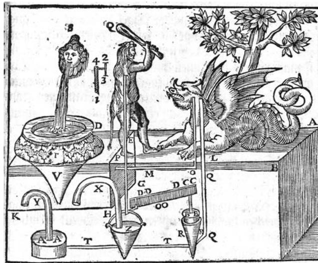
When the human figure is turned toward the dragon, a valve between the two sealed chambers under the figure closes. However if the human figure is rotated to the side, the valve connecting the two chambers opens, water flows from the top to the bottom chamber, and suction is created in the pipe leading from the upper chamber to the dragon's mouth. Because of this suction, the dragon appears to drink if a cup of water is held up to its mouth. (Buch von Luft-Und Wasser-Kunsten, page 3)
