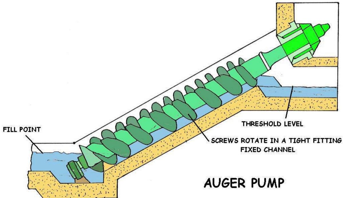
The machine consists of a screw inside a hollow pipe. Some attribute its invention to Archimedes in the 3rd century BC, while others attribute it to Nebuchadnezzar II in the 7th century BC. A screw can be thought of as an inclined plane (another simple machine) wrapped around a cylinder.
