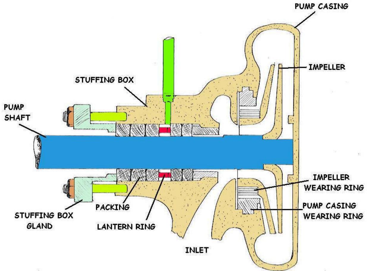
A centrifugal pump has two main components:
