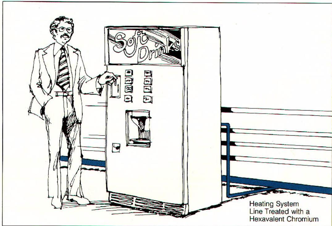
***Several cross-connection have been made to soda machines, the one to worry about is when you have a copper water line hooked to CO<sub>2</sub> without a backflow preventer. The reason is that the CO<sub>2</sub> will mix in the water and create copper carbonic acid, which can be deadly. This is one reason that you will see clear plastic lines at most soda machines and no copper lines. Most codes require a stainless steel RP backflow assembly at soda machines.***
