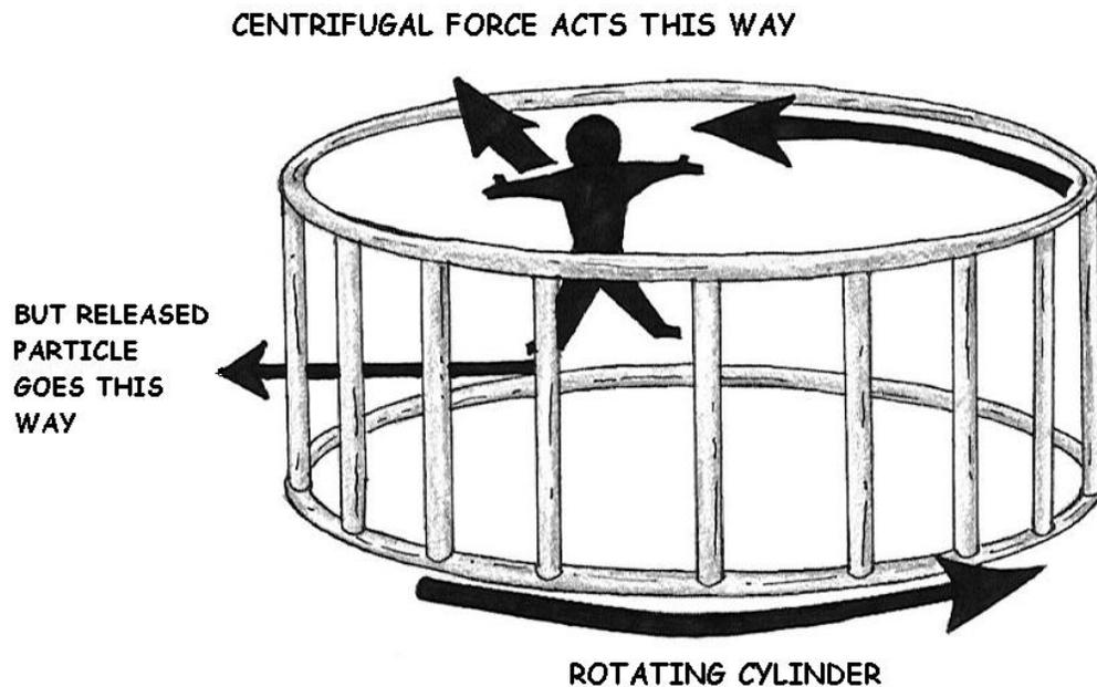
First, you can view the water between the impeller blades as an object traveling in a circle. Objects do not naturally travel in a circle--they need an inward force to cause them to accelerate inward as they spin.
