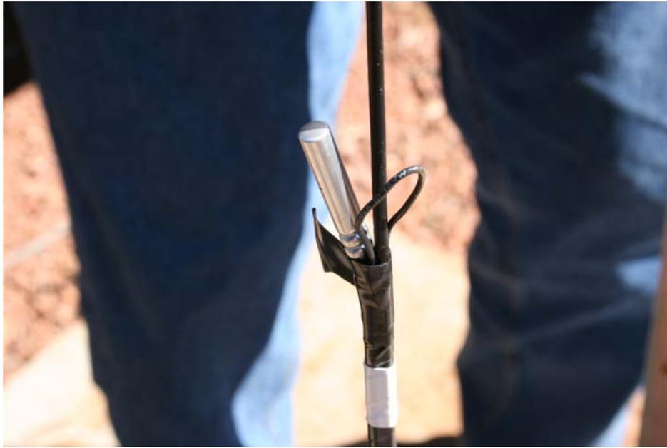
**Blasting cap on the explosive cord. Below, some of the debris from inside the well casing following the explosion. After talking to this man, I found out that after 9-11, he had to increase his fees because of the ATF and new rules concerning explosives. Be prepared to pay through the nose for this treatment process. Consider this expense the price of admission to having adequate water to supply your customer's demands.**
