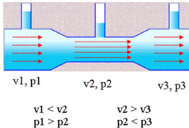
After the first venturi the pressure in the pipe is lower, so the gas is sucked in the pipe. Then the mixture enters the second venturi and slow down. At the end of the system a mixture of gas and liquid appears and the pressure rise again to its normal level in the pipe. This technique is used for ozone injection in water.
