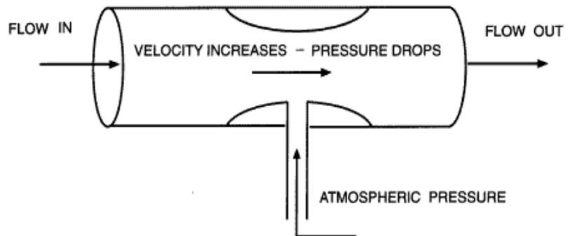
The newest injector design causes complete mixing of injected materials (air, ozone or chemicals), eliminating the need for other in-line mixers. Venturi injectors have no moving parts and are maintenance free. They operate effectively over a wide range of pressures (from 1 to 250 psi) and require only a minimum pressure difference to initiate the vacuum at the suction part. Venturis are often built in thermoplastics (PVC, PE, PVDF), stainless steel or other metals.
