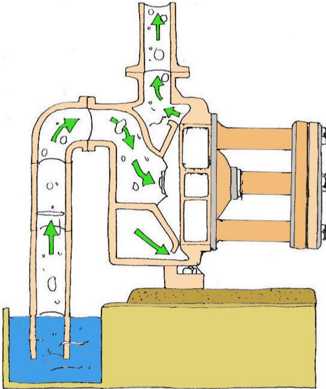
**Self-priming pump:** A pump that does not require priming or initial filling with liquid. The pump casing carries a reserve of water that helps create a vacuum that will lift the fluid from a low source.
