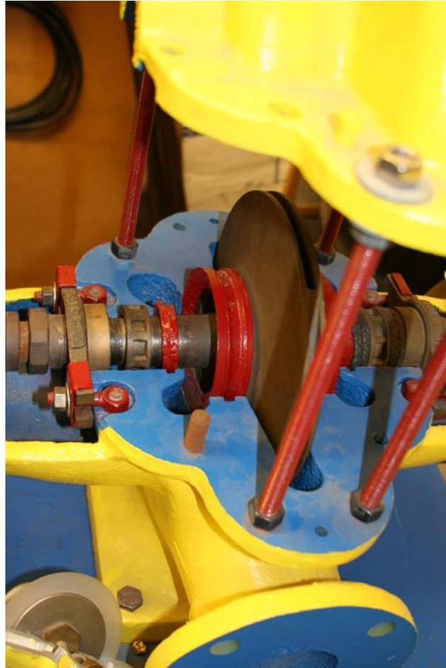
**Lantern ring:** A metal ring located between rings of packing that distributes gland sealing fluid. You can see that one side of the shaft is missing packing for the lantern ring.
