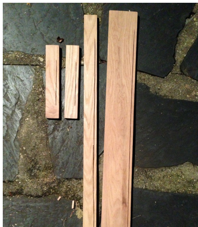
Ridges cut into the aprons for the table top fasteners. I used a circular saw so it was difficult.
