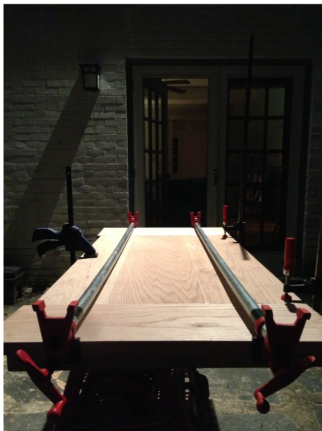
The two end pieces joined. The pipe clamps are bending but I fixed that after I took the picture.
