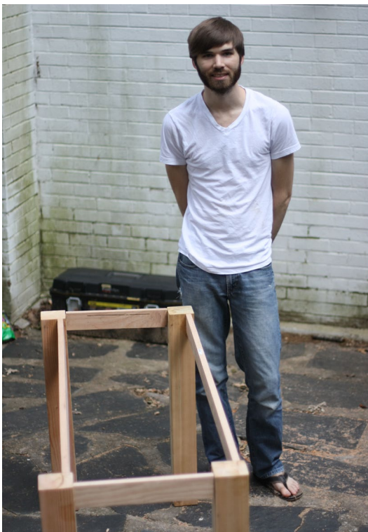
The final base. The left apron is on the inside because it will have a ledge to hold all the cords in the back.
