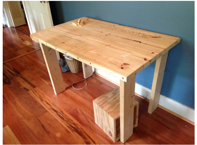
My first prototype wooden desk. Learned how to glue boards together and drill dowel holes. Without aprons, it wobbled.
