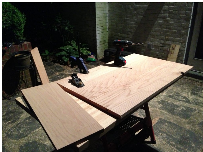
Joining the two end pieces. You can see the dowel holes.
