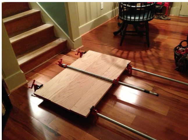
The boards were connected with dowels (using a doweling jig to drill the holes) and a bunch of wood glue, and clamped with pipe clamps.
