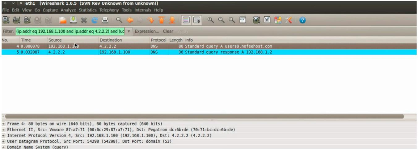
Figure 13. Wireshark showing DNS query made by the malware
