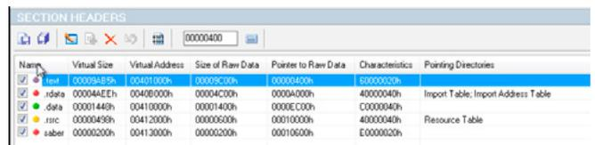
Figure 8. View file sections using PE Explorer
