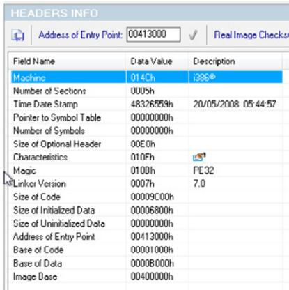
Figure 6. Viewing file header information using PE Explorer
