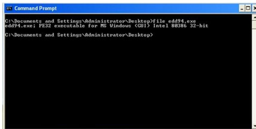
Figure 4.5: file utility showing executable file
