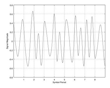
Figure 3.2. Amateur Bell 202 signal representing the ASCII letter A (0x41)
