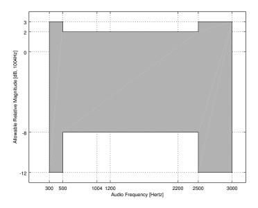
Figure 3.7. Allowable skew in a basic 3002 telephone channel
