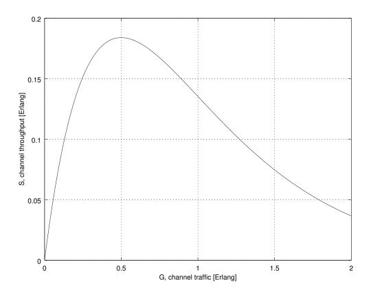
Figure 8.1. Poisson channel traffic and throughput
