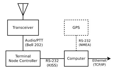
Figure 2.4. Block diagram for typical APRS Internet Gateway
