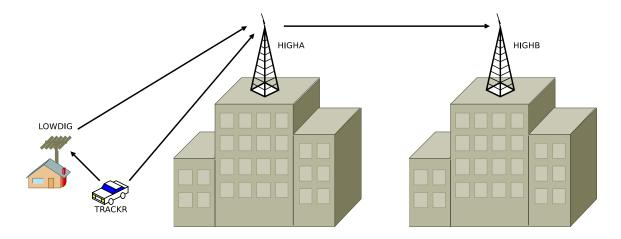
Figure 6.1. APRS network used for path routing examples
