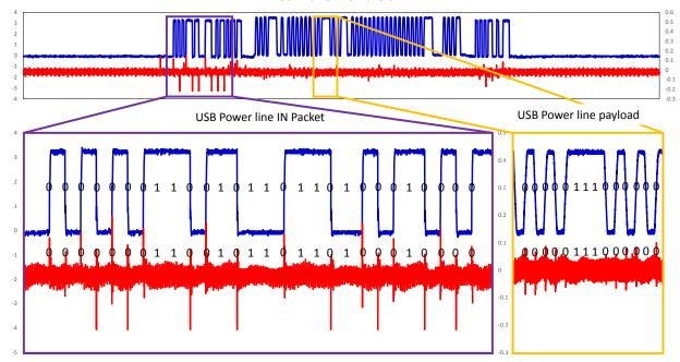
Figure 13: USB communication (blue, top) and power line crosstalk leakage (red, bottom) of a single 1ms USB frame with a keyboard attached to the USB hub. The data line crosstalk leakage was captured using the hub from Figure 7(rightmost).
