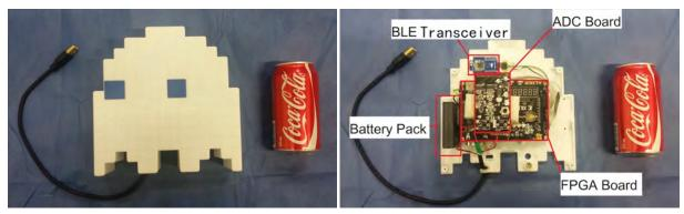
Figure 21: The external appearance of the spy probe, which is embedded inside a toy ghost lamp, size is compared with a 375mL classic Coca-Cola can (left). Inside look of the spy probe, showing the ADC board, FPGA board, BLE board and battery pack (right).
