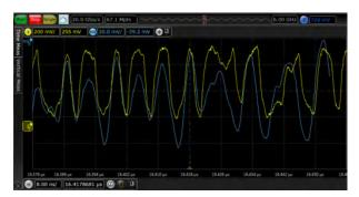
Figure 10: USB 2.0 data line crosstalk leakage from a hub of the same make as the one used in Figure 6. The yellow (top) trace shoes the USB traffic and the blue (bottom) trace shows the observed data line crosstalk leakage measured from an adjacent downstream port (manually aligned with the yellow trace by subtracting 4ns).
