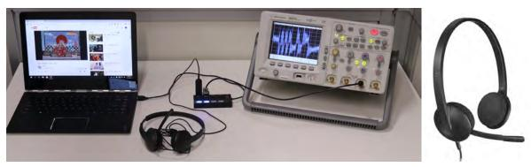
Figure 18: (left) Experimental setup for observing data line crosstalk leakage from a USB headset microphone (Logitech H340). The data line crosstalk leakage is clearly visible on the oscilloscope's screen. (right) Logitech H340 USB headset.
