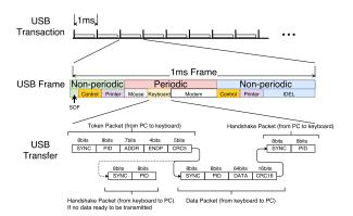
Figure 2: USB transaction, frame and packets.
