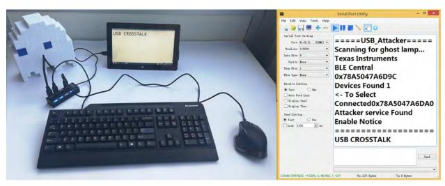
Figure 23: Demonstration of our attack. (left) Phrase being typed on the Surface Pro via a USB keyboard. (right) extracted key presses corresponding to the string "USB CROSSTALK".
