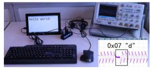
Figure 15: Extracting keyboard presses using data line crosstalk leakage. The scan code 0x07 corresponding to the letter d is clearly visible in the leakage trace.
