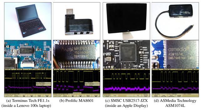
Figure 4: Top and middle row: Four tested USB hubs and their controller chips found to contain data line crosstalk leakage. Bottom row: Corresponding leakage waveform, yellow (top) trace shows the USB traffic and purple (bottom) trace shows the data line crosstalk leakage measured from an adjacent downstream USB port.
