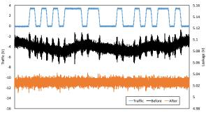
Figure 26: Evaluation of our USB condom showing the actual USB communication (blue), the corresponding unmitigated power line crosstalk leakage (black) and the power line crosstalk leakage measured on the USB port of our USB condom (orange). Notice that the power line crosstalk leakage is significantly attenuated.
