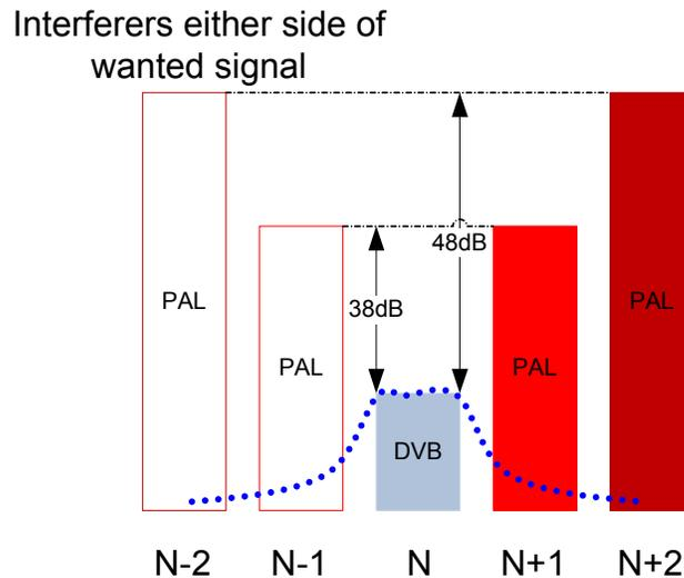
Figure 8: Channel of Interest with Adjacent Channel Interferers
