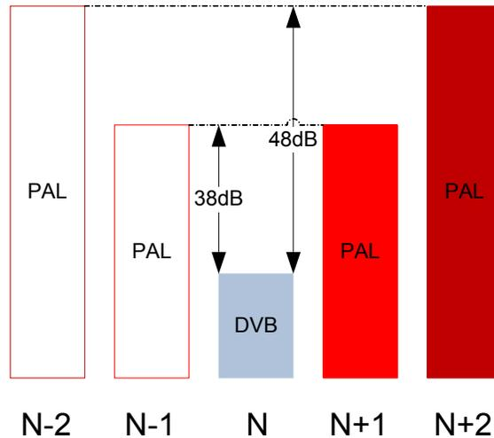
Figure 6: Channel of Interest with Interferers
