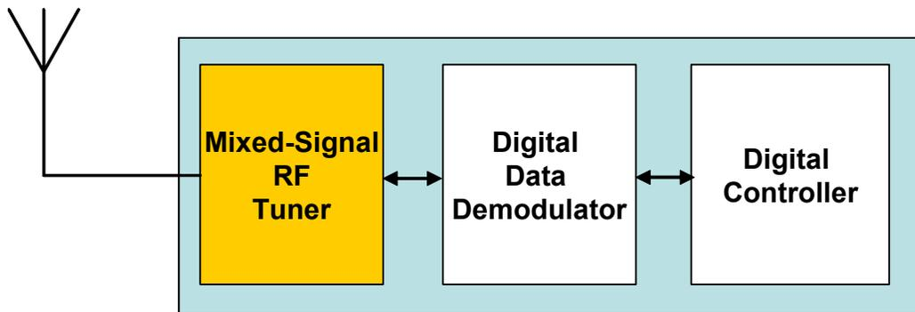
Figure 4: Digital Receiver Architecture
