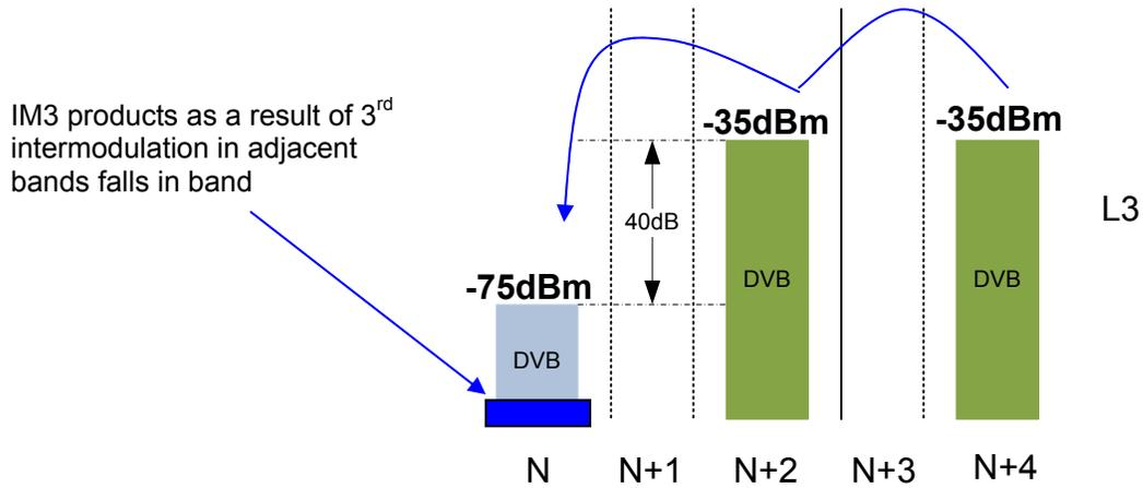
Figure 7: Channel of Interest with Alternate Channel Interferers
