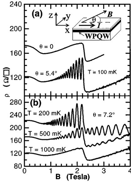
FIG. 1. (a) Magnetoresistivity traces for  $\theta=0$  (upper curve, displaced upward by  $50 \Omega$  for clarity) and  $5.5^\circ$  (lower curve). Inset: WPQW sample, showing  $B$  tilt orientation. (b) Temperature dependence of the oscillations for a fixed tilt of  $7.2^\circ$ , again offset for clarity.
