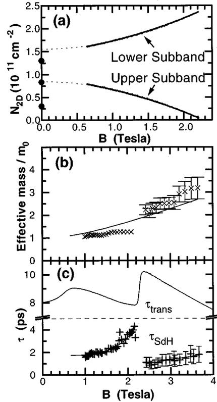
FIG. 3. Electron properties in the WPQW, as a function of electric field: (a) Electron sheet densities in the lowest- and second-lowest subbands; circles at  $B_x=0$  are from fast Fourier transform data where  $B_x\parallel z$ . (b) Electron effective mass, normalized such that the effective mass in GaAs ( $0.067m_e$ ) corresponds to 1; (c) electron scattering times— $\tau_{SdH}$  derived from SdH data and the mobility-determined scattering lifetime  $\tau_{trans}$ .
