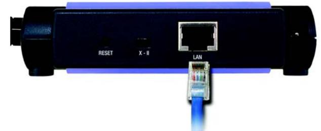
Figure 4-1: Connect the Ethernet Network Cable
