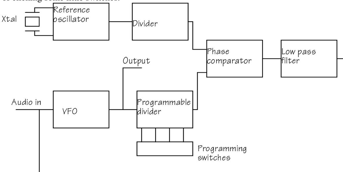
Hang on a sec, the VFO is being frequency modulated by the audio input, so its frequency at any given instant depends on the voltage of the audio output. We don't want this variation of the VFO's frequency to be ironed out by the PLL system, so we 'iron out' the error voltage from the phase
