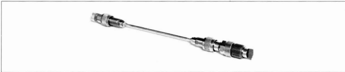
Figure 88 Photograph of DUT No. 2 with N connectors and 50 \Omega termination (left)
