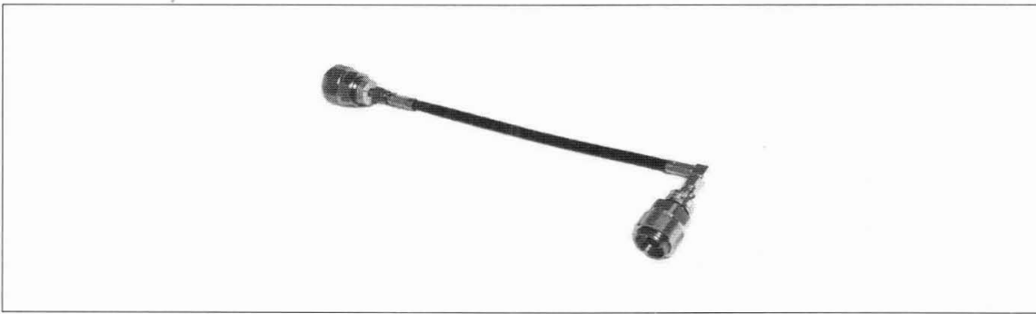
Figure 85 Photograph of DUT No. 1 with SMA connectors and the test port adaptors (SMA-PC7)
