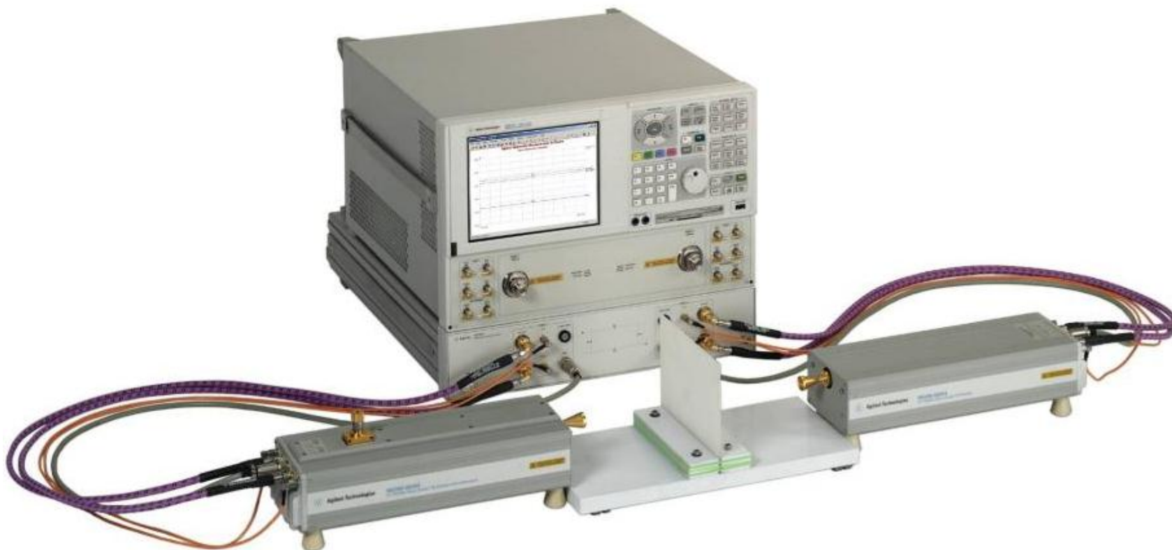
Dielectric measurement setup for free space measurement
