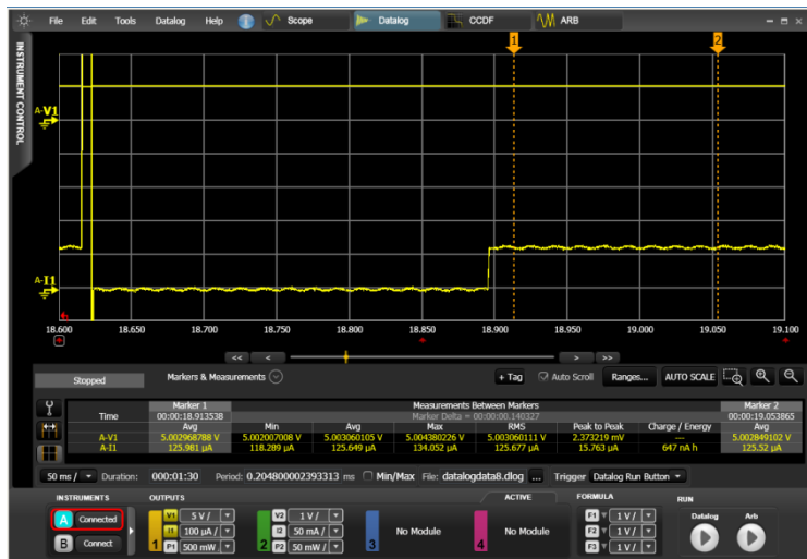
Figure 17: Looking a \mu A-level sleep current signal between pulses in data log mode
