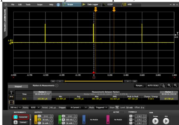
Figure 7: 14585A Determining Pulse Valley Values Using Markers
