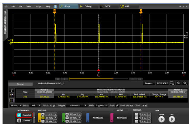
Figure 5: 14585A Pulsed Current Drain Waveform Acquisition
