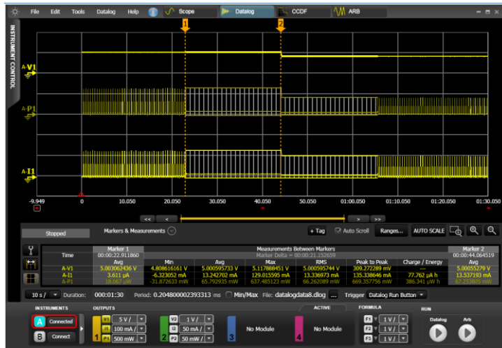
Figure 16: Power trace and vertical markers turned on
