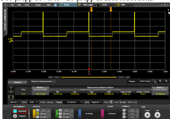
Figure 9: Expanding the Pulse Valley Amplitude, Seamless Ranging Measurement Turned On
