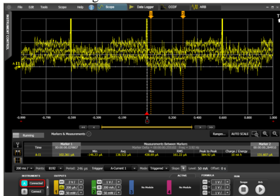
Figure 8: Expanding the Pulse Valley Amplitude
