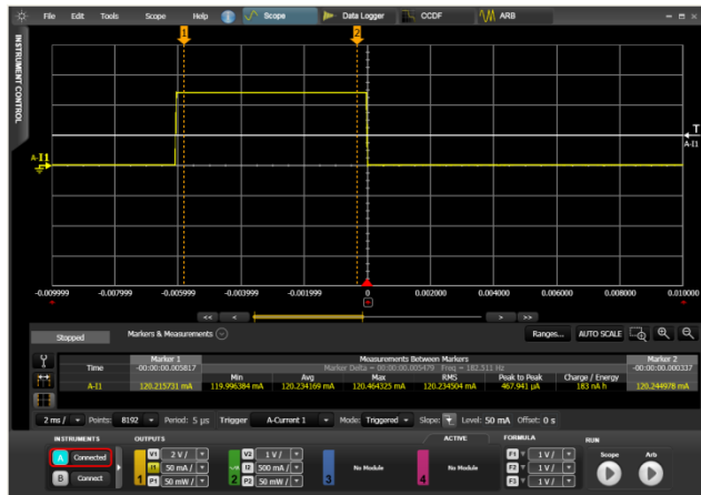
Figure 6: 14585A Determining Pulse Plateau Values Using Markers
