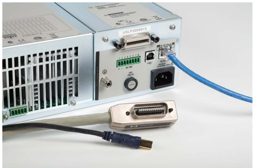
Figure 3: Built-in ethernet, USB 2.0, and GPIB interfaces enables easy system connections
