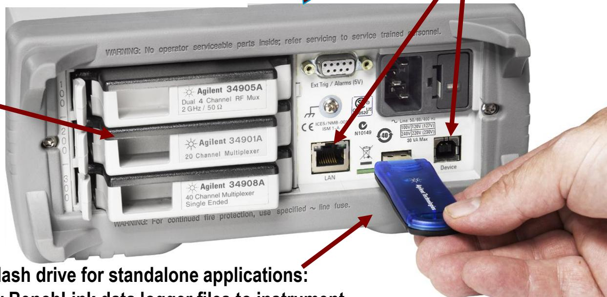
Choose from 8 plug-in modules with on-board screw terminals
