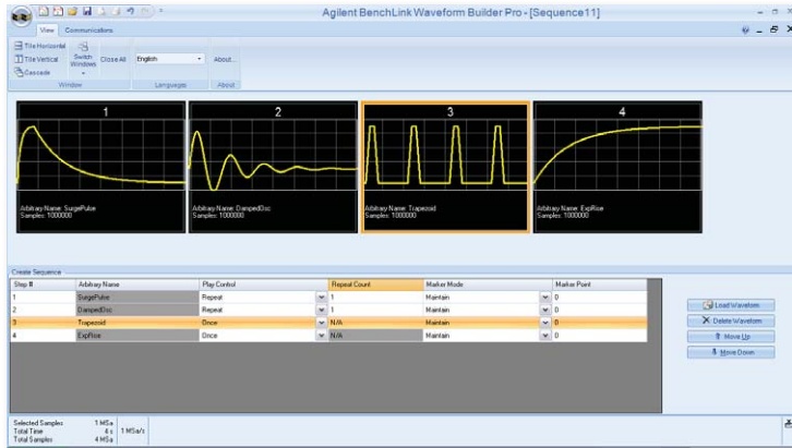
Figure 2. Arbitrary Waveform Sequences: Use the Waveform Sequence Tool to create longer custom waveforms by linking multiple waveforms together.
