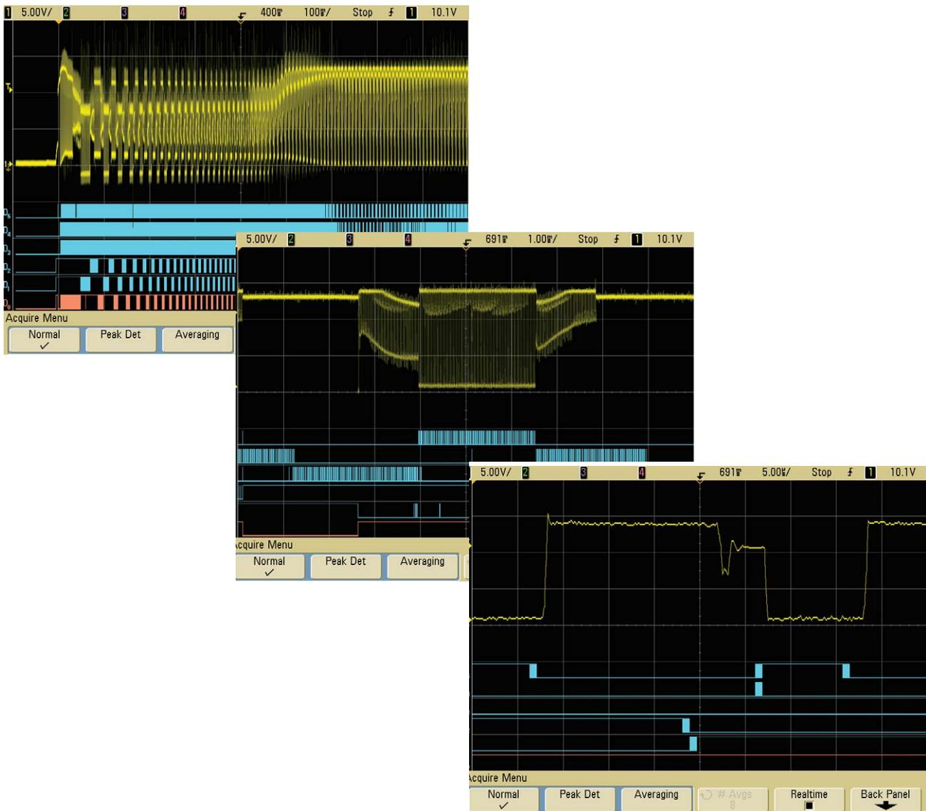
**MegaZoom III deep memory helps you find details buried in complex signals. You can view fast waveform updates of signals by means of an external display connected to the oscilloscope's XGA out port.**
