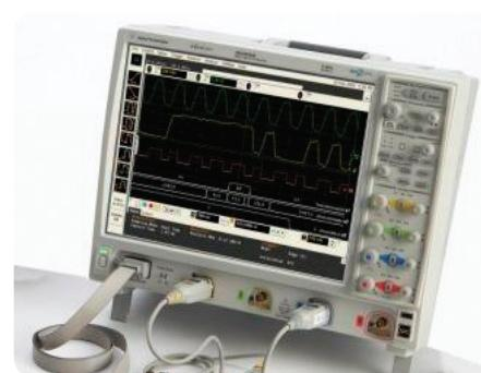
Integrated mixed-signal oscilloscope lets you trigger across time-correlated analog and digital channel combinations.
