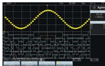
2000 X-Series' exclusive MSO adds eight integrated digital channels for extra triggering or logic analysis; DSO models are customer-upgradable to MSO models
