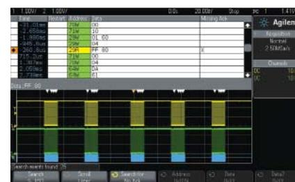
3000 X-Series protocol-aware triggering, decode, search, and navigation for serial buses; hardware-based to maintain fast waveform update rate and capture elusive errors
