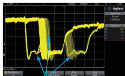
Infrequent glitches and signal jitter captured after 1 second on 3000 X-Series with > 1,000,000 wfms/s
