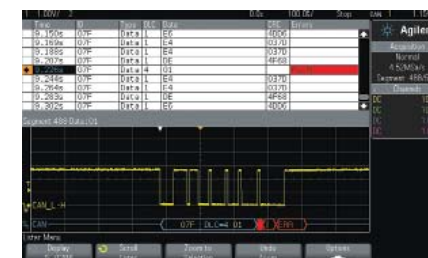
500 CAN serial packets over 9 seconds, captured at a high sample rate, using the 3000 X-Series's segmented memory
