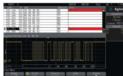
Infrequent LIN bus parity error captured on the 3000 X-Series in less than a second due to hardware-based serial decode
