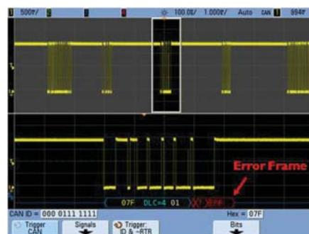
Turning on serial decode on Agilent's InfiniiVision 7000B has no impact on its waveform update rate and it is able to capture the error frame on this CAN bus
