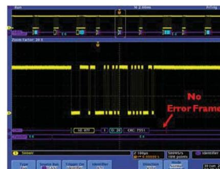
Turning on serial decoding severely limits the update rate of the Tektronix 4000 series as it is not able to capture the error frame
