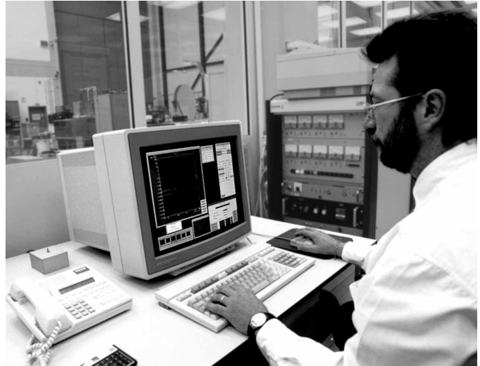
Figure 2: The m+p VCP9000 System The m+p VCP9000 vibration control system is built around HP 3565S measurement hardware with m+p VibControl software.
