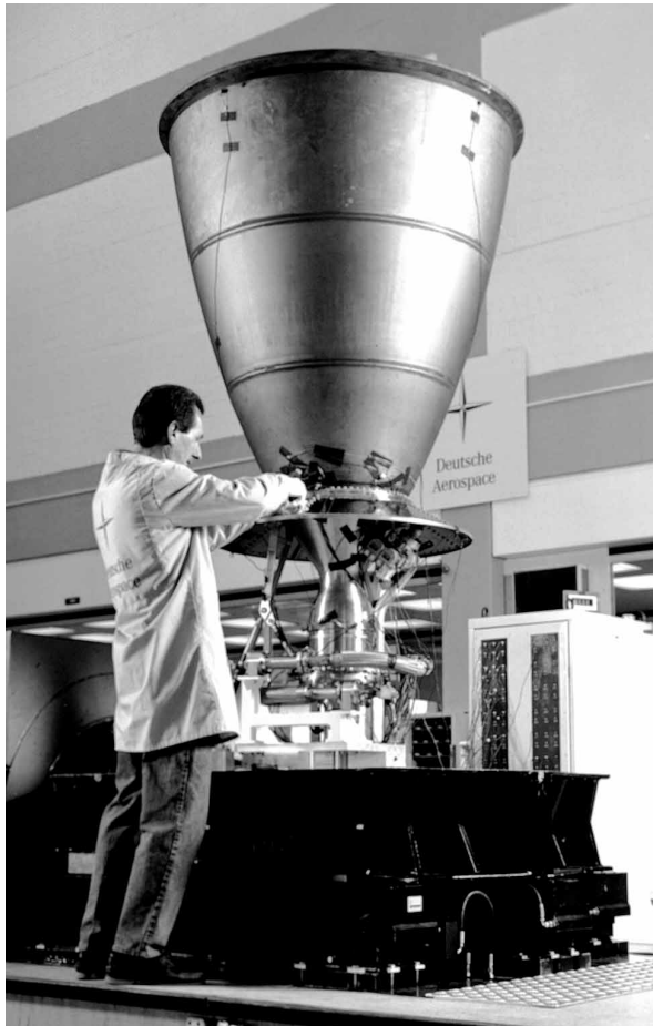
Figure 1 Subsystem Tests A Deutsche Aerospace specialist prepares a test of the AESTUS engine for the European launch rocket ARIANE V.
