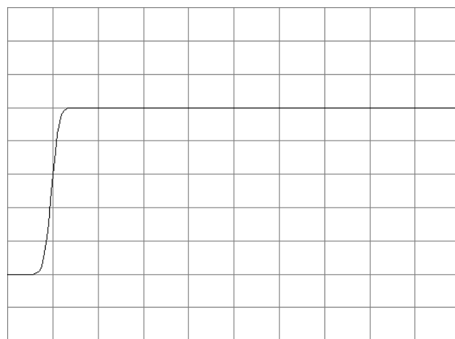
Figure-14, Step response of 4 MHz analog alias filter with 12-tap compensation giving a Gaussian response with 1 MHz 3 dB bandwidth. Horizontal scale is 1 \mu s/div.
