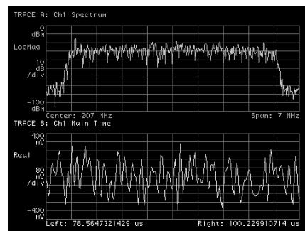
**HP 89400 vector signal analyzers also provide a complete set of traditional spectrum and waveform measurements.**
