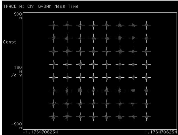
**64QAM signal analysis accommodates differential encoding for DVB systems, as well as absolute encoding.**
