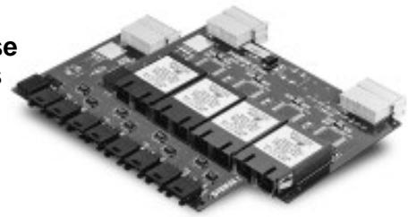
The multi-speed, general-purpose, 4-port NTS port card is designed to operate with signals of any encoding or baud rate (up to 1 GHz) from any electrically compatible Fibre Channel transceiver. There is no retiming circuitry. This allows the port cards to operate with a wide range of baud rates and various types of encoders such as SMPTE video, SONET, and FDDI. Port cards are available for both non-OFC short wave laser or copper connections.
