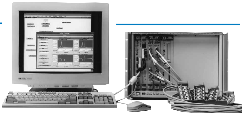
The HP E3203A Measurement Engine supports the new HP E1432A 16-channel digitizer.
