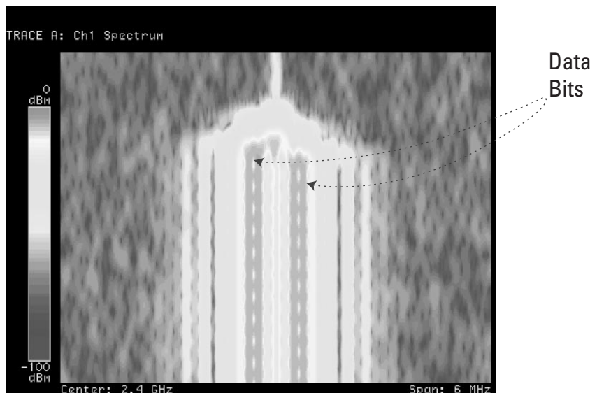
Figure 17. HP 89441A spectrogram display for symbol timing and rate
